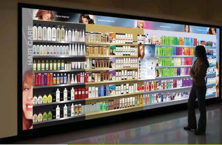
P&G's 'virtual wall' uses multiple projectors to simulate store shelves for faster consumer testing.
