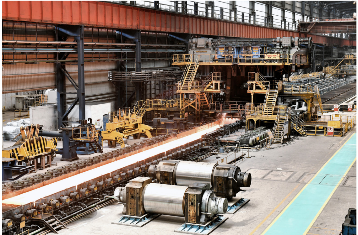
The hot strip mill makes coils of various types of steel, producing around 5.5 million tonnes per year.
